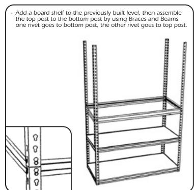
Add a board shelf to the previously built level, then continue by adding the last two levels of beams and braces to the unit.
